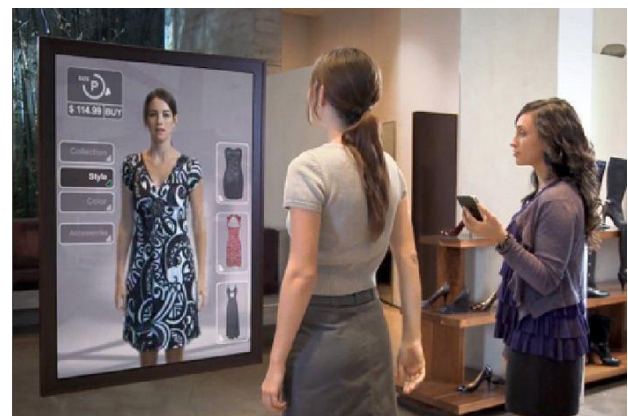
Figure 5. AR system using spatial displays
